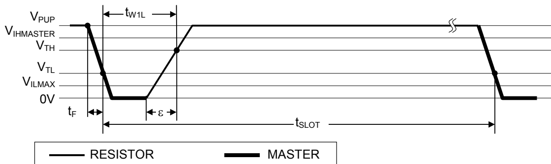
Figure 16. Read/Write Timing Diagram
