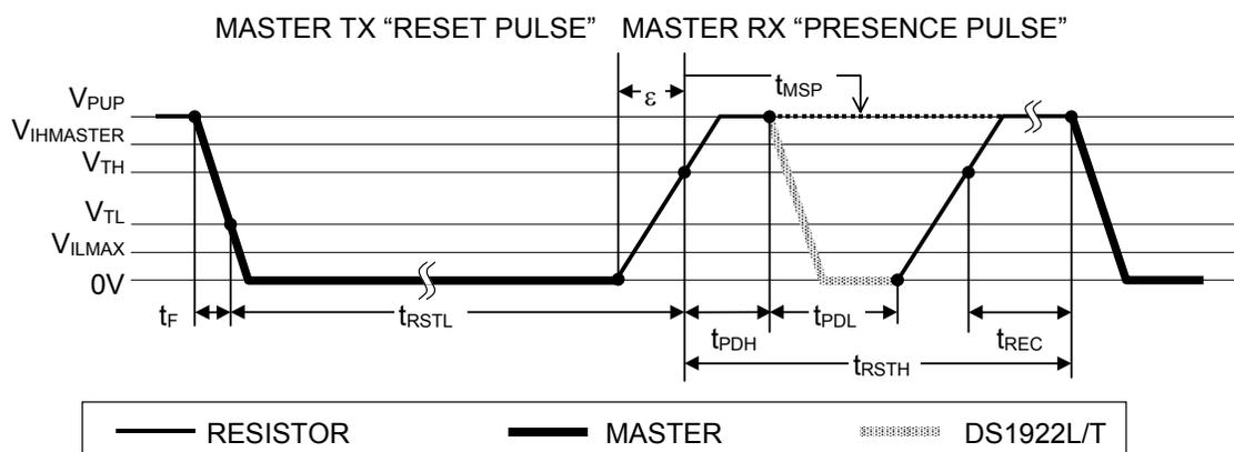
After the bus master has released the line it goes into receive mode (RX). Now the 1-Wire bus is pulled to  $V_{PUP}$  through the pullup resistor or, in case of a DS2480B driver, by active circuitry. When the threshold  $V_{TH}$  is crossed, the DS1922L/T waits for  $t_{PDH}$  and then transmits a presence pulse by pulling the line low for  $t_{PDL}$ . To detect a presence pulse, the master must test the logical state of the 1-Wire line at  $t_{MSP}$ .
