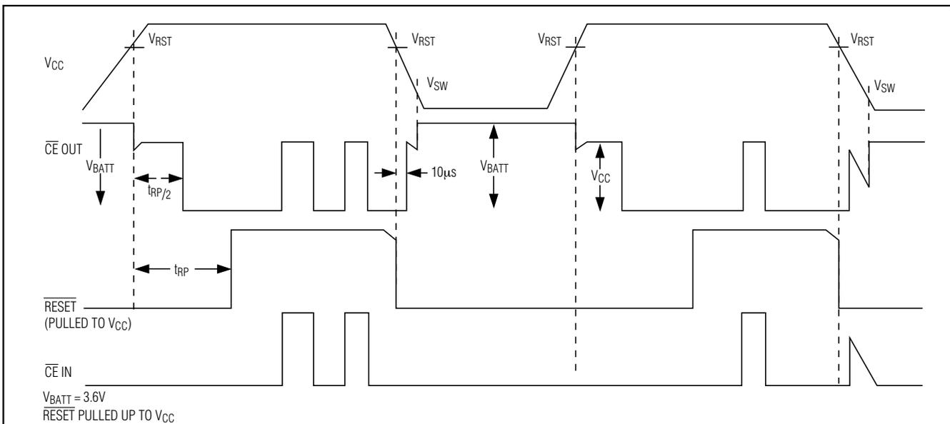
Figure 8. Chip-Enable Timing
