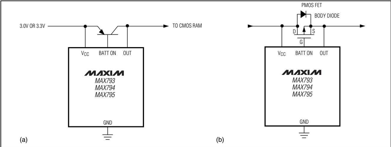
Figure 14. Driving an External Transistor with BATT ON
