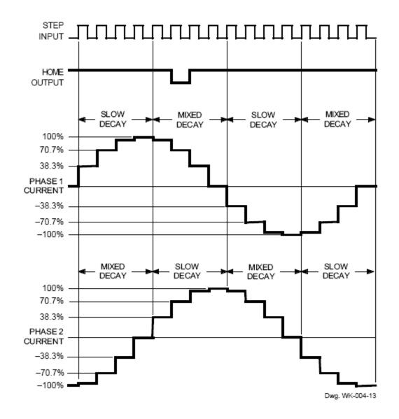
The mixed-decay mode is controlled by the percent fast decay voltage (V<sub>PFD</sub>). If the voltage at the PFD input is greater than  $0.6V_{DD}$  then slow-decay mode is selected. If the voltage on the PFD input is less than  $0.21V_{DD}$  then fast-decay mode is selected. Mixed decay is between these two levels.
