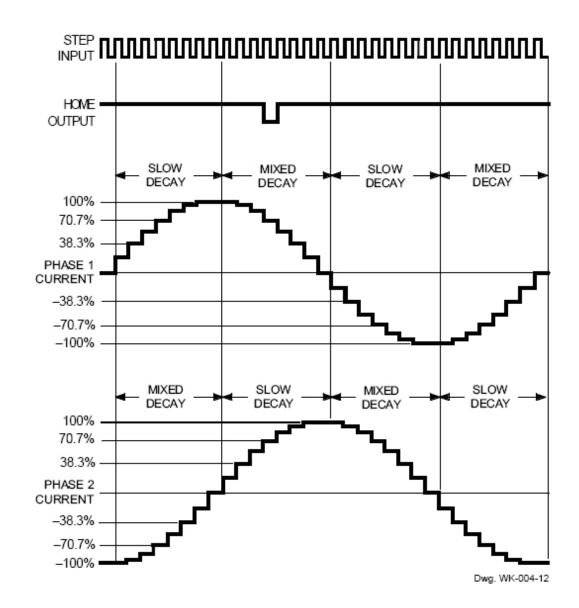
The mixed-decay mode is controlled by the percent fast decay voltage ( $V_{PFD}$ ). If the voltage at the PFD input is greater than 0.6V<sub>DD</sub> then slow-decay mode is selected. If the voltage on the PFD input is less than 0.21V<sub>DD</sub> then fast-decay mode is selected. Mixed decay is between these two levels.
